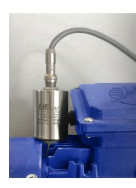
The UltraTrak 850 sensor requires a KCF Technologies IoT Hub and analog adapter for use.
