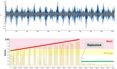
Continuous, live-feed vibration monitoring reveals underlying fault conditions in real time.
